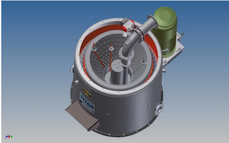
Figure 3. Titan 1300 "A" massecuite configuration top view
