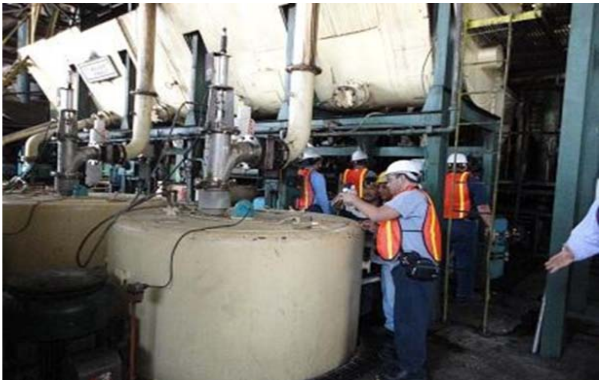
Figure 4. Titan 1300 "B" or "C" massecuite configuration
