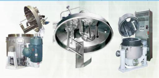
The Quadramatic is a vertical, bottom discharging or top unloading centrifuge developed to generate up to 2,000 gravities of separation force. When operated as a filtering centrifuge, Quadramatic centrifuges can remove most if not all of the unbound moisture without the need for thermal processing to deliver a cost-effective and dependable method of separating solids and liquids for medium to full scale production.
